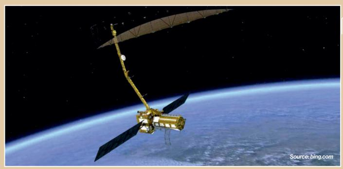
The NASA-ISRO Synthetic Aperture Radar (NISAR).
