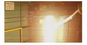
version of their patented technology based single piece, fully 3d printed, 2nd stage semi cryo engine – Agnilet – at VSSC, ISRO
